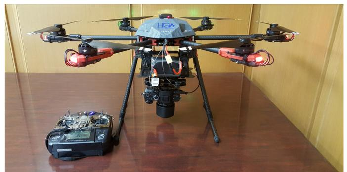
collection information is streamed to the ground station from all aircraft utilizing on board telemetry radios. Using reliable, customized UAVs, we can vastly reduce the time spent collecting accurate data, resulting in more accurate project plans, models and operations.
